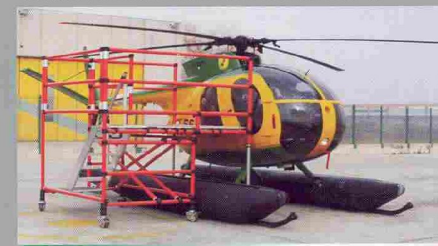
NH 500 uni-tec main and tail rotor access staging
