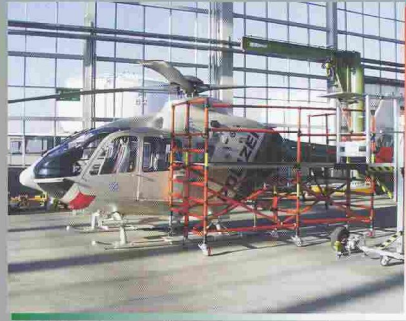
AEC 135 uni-tec main rotor access staging
