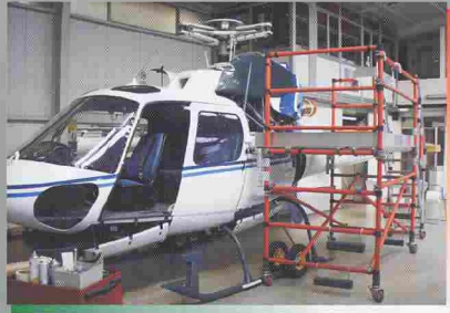
ECUREUIL uni-tec main rotor access staging
