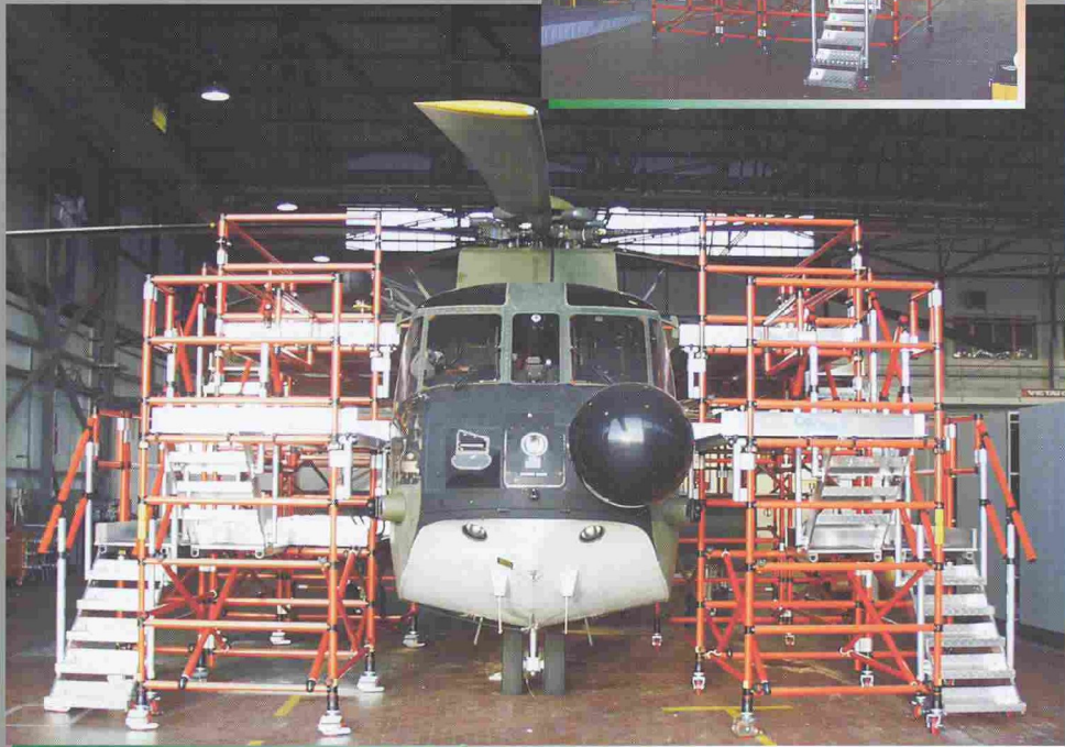
HH3F uni-tec full access staging
