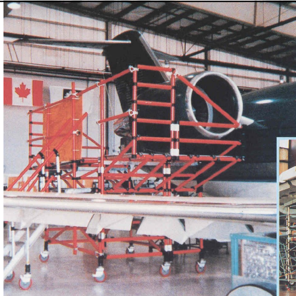
UNI-TEC structure with overhang for Challenger 604 engine maintenance
