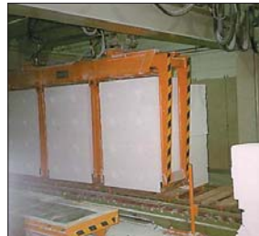
Cube Clamp STAZ with Hydraulic Divider
