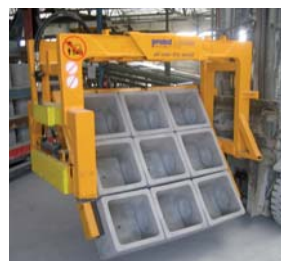
Fork Lift Grab STAZ with 180° rotating grippers
