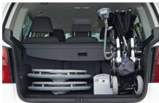
The powered wheels without stud axles make storage particularly easy and space-saving
