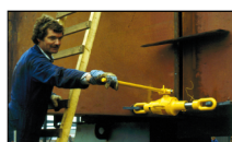
PL 2510 being used to pull ship sections together
