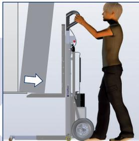
Push load onto the fork-plate.
