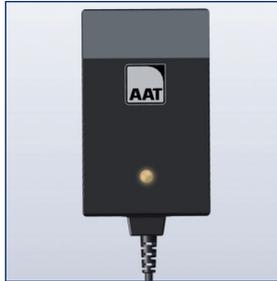
LED orange = batteries are being charged
