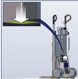
Release the locking mechanism and remove the battery pack.
