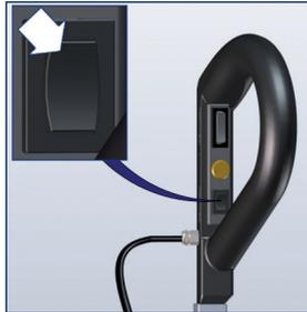
Press lift function UP/DOWN direction **UP**, until the fork-plate is approximately 10 mm underneath the edge of loading area.
