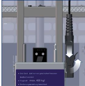
Put helix cable into its socket and lock it.
