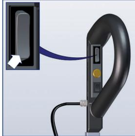
Press UP/DOWN switch direction **DOWN**.
