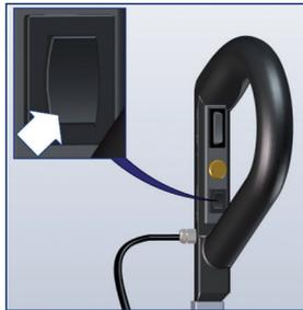
Press lift function UP/DOWN direction **DOWN**, until the fork/toe-plate reaches its neutral position (see chapter 4.6).
