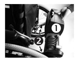
Please insert the max-e with its wheelchair connections 1 in a straight line in reference to the brackets 2.
