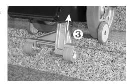
Because the s-max is always pulled slightly backward, it rolls automatically to the next step and reaches the initial position again - both main wheels touch the next step  ${\bf 0}$ .
