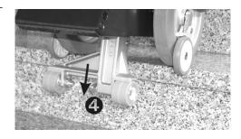
When the climber reaches the next lower step  $\mathbf{G}$ , it resumes the load of the main wheels, while those plus the climbing frame are lifted off the higher step  $\mathbf{G}$ .
