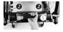
$^{\circ}$  Make sure the v-max with its wheelchair links lacktriangle is in a straight line when you insert it into the brackets lacktriangle.
