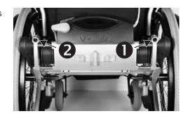
If you like, remove the v-max entirely from the wheelchair and set the device on its grips, which function as sturdy legs in such case.
