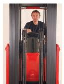
Operators have excellent forward visibility thanks to the triplex free lift mast, with its twin side mounted lift cylinders. Mast tilt means easy fork entry into pallets – even over trailer retaining raves.
