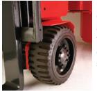
Four large cushion rubber tyres deliver optimum performance and traction in loading yard. They're also resistant to damage which means a long service life and less downtime.
