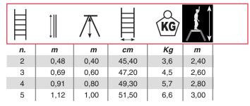
European standard UNIEN14183: with PUNTO S 2 and 3 steps the operator can stand on the last steps or on the platform even without a guardrail (optional). A 60 cm guardrail is mandatory only for the 4th and 5th steps.
