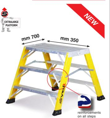
Stepstool with insulating dielectric fiberglass stiles and aluminum steps. Double sided it is equipped with an extra large platform to stand comfortably and safely at maximum height. Equipped with steel safety rods. Each step is reinforced with galvanized steel bars.
