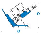
\* The metric equivalent of working height adds 2 m to platform height. U.S. adds 6 ft
