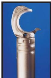
**Self - locking hook** in aluminium castings click easily into position on the tubular frame. Segmental latches give more than 225° contact area ensuring maximum tower stability. The hooking edge is reinforced to make it shock-proof. Brace model and length are printed on the casting to easily identify this detail.
