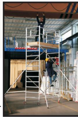
**Jolly 6.27m (Modules A+B+C+D):** The extension D include an additional complete platform and 2 guardrails for a working height of 7.22m (Platform Height 5.22m). (A+B+C+D = only 36 components – 155 Kg).
