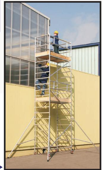
Starting from the height of 4.47 m (Platform Height 3.42m) onwards, it is possible to mount Modules D (with platforms and guardrails) and E in order to reach a maximum height of 11,67 m (Platform Height 10.62m). The tower's frames can safely be used as ladders for climbing (rung distance 30 cm) minimising components required for storage.
