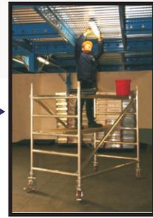
**Jolly 4.47 m (Modules A+B+C):** Adding the guardrail section B which includes 2 frames and 2 guardrails, and the extension C which includes 4 stabilisers (compulsory over this height) Jolly can be assembled to a total height of 4.47m (Platform Height 3.42m). (A+B+C = only 24 components – 108 Kg).
