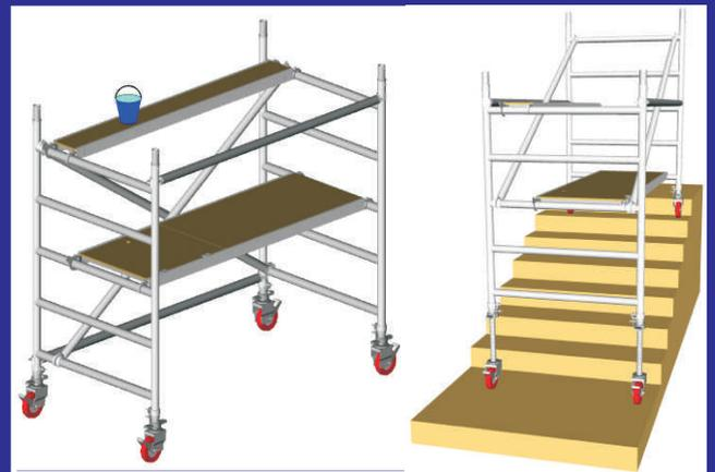
Module A of the Jolly tower system is 1.81 m high and allows a maximum working height of 3.00 m. It can be transported erected through standard door widths and also can be used on stairwells. Overall dimensions are 2.00 m x 1.05 m
