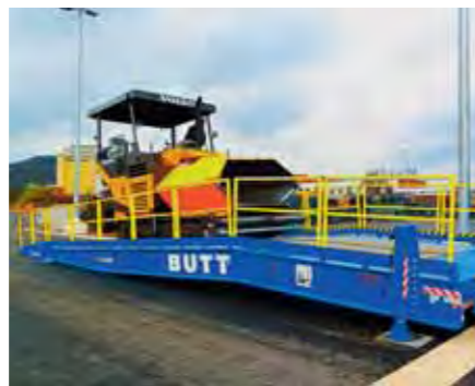
Construction vehicle loading up to 4 m drive width and 35 t carrying capacity.
