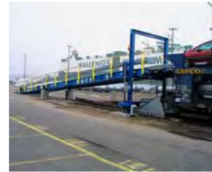
Passenger car double-decker rail loading.
