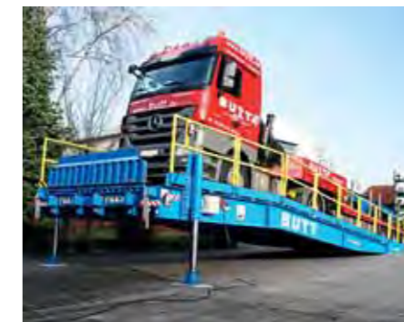
Lorry loading with electrohydraulic height adjustment.
