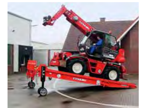
Short mobile ramp for loading construction vehicles.
