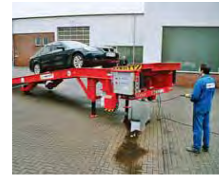
Mobile yard ramp with dock leveller and electric end carriage.
