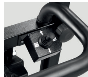
Joystick control on the fixed handle
