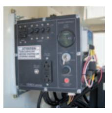
Control box shown with optional Roda Deaco electronic air shutdown system (model AL5000).
